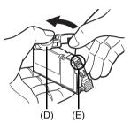
(D) Carefully hold the protective cap when removing it to prevent the ink from staining your fingers. Install the ink tank.
